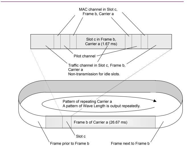
Figure 3.1.5.1-3 Image of 1xEV-DO forward single carrier waveform pattern repetition
