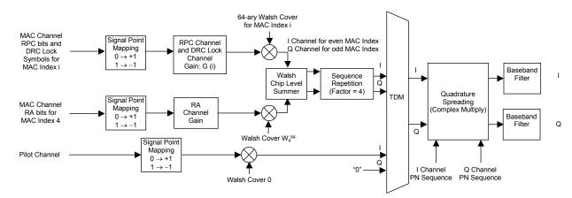
Figure 3.1.5.1-5 Block diagram of 1xEV-DO forward idle slot
